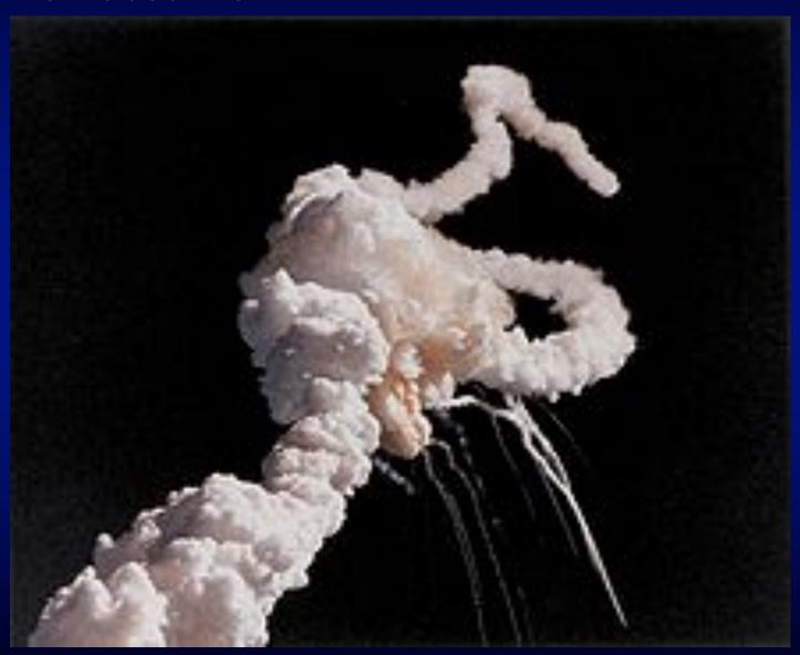
In 1986, the *Challenger* was destroyed during launch because of a faulty O-ring design that could not handle the freezing temperatures of the previous night
